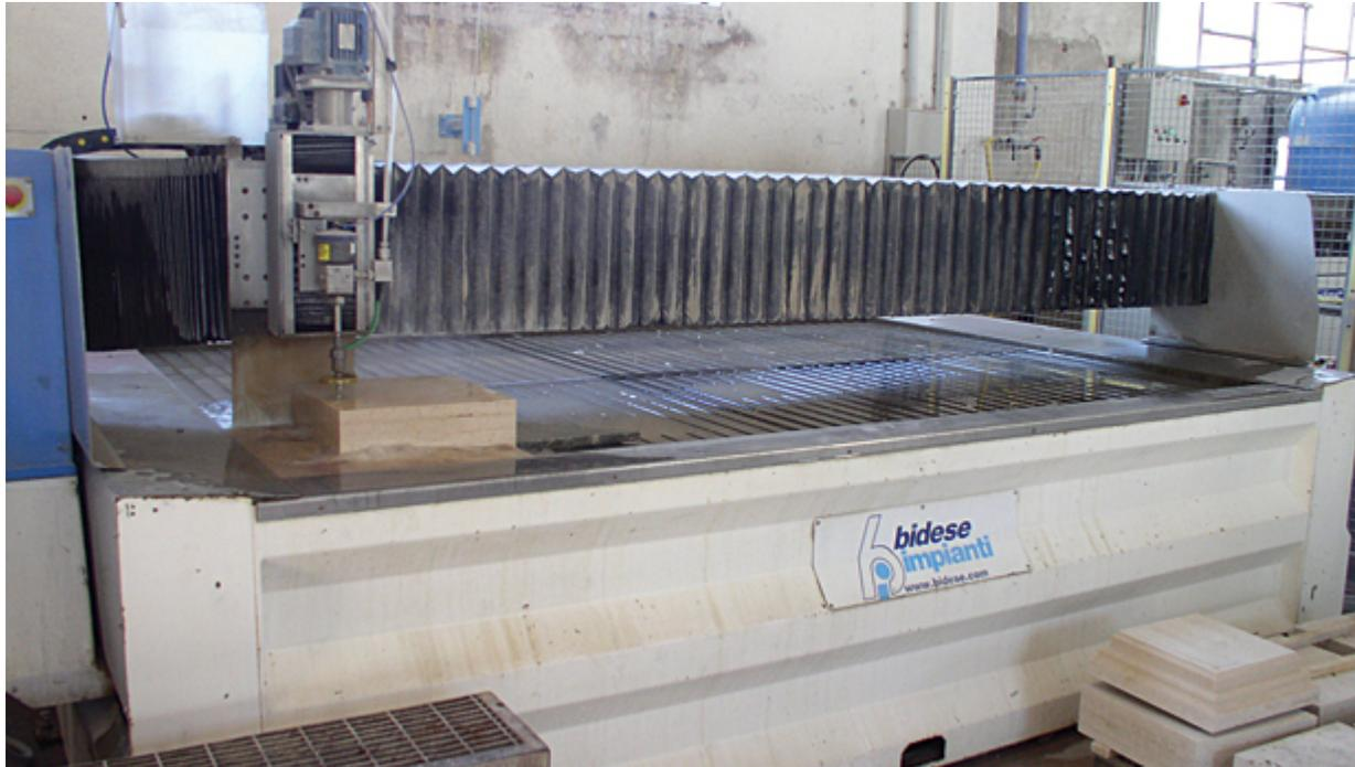
Complex cutting is achieved using two waterjets, including a Bidesimpianti model from Italy.
